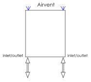
Vertical mount All Dimensions are in mm Max.Working Pressure: 10 Bar Max.Working Temperature: 95° C Inlet / Outlet: 1/2" BSP Fuel: E/H/D
